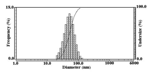
Figure 2: PSA of CuO-water nano-suspensions PVP surfactant.
