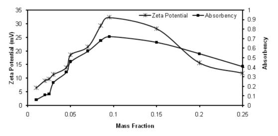
Figure 5: Effect of PVP concentration on the zeta potential and absorbency of CuO-water.
