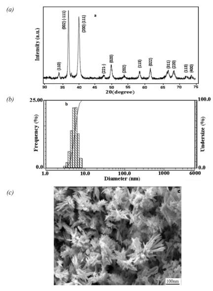
Figure 1: (a) XRD pattern, (b) PSA pattern, and (c) SEM pattern of CuO nanoparticles.
