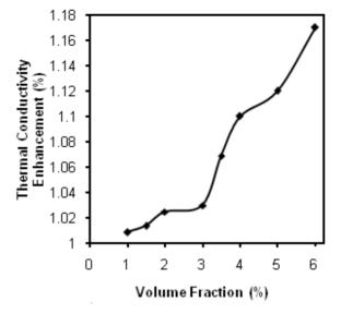
Figure 6: Effect of volume fraction CuO nanoparticles on the thermal conductivity of nano-suspensions with PVP surfactant.
