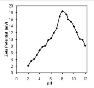
Figure 3: Effect of pH on the zeta potential of CuO-water nano-suspensions with PVP surfactant.
