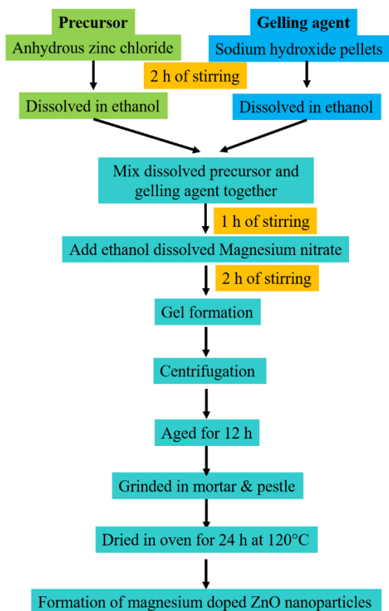
Figure 1. Schematics of sol-gel mediated magnesium-doped ZnO nanoparticles synthesis.
