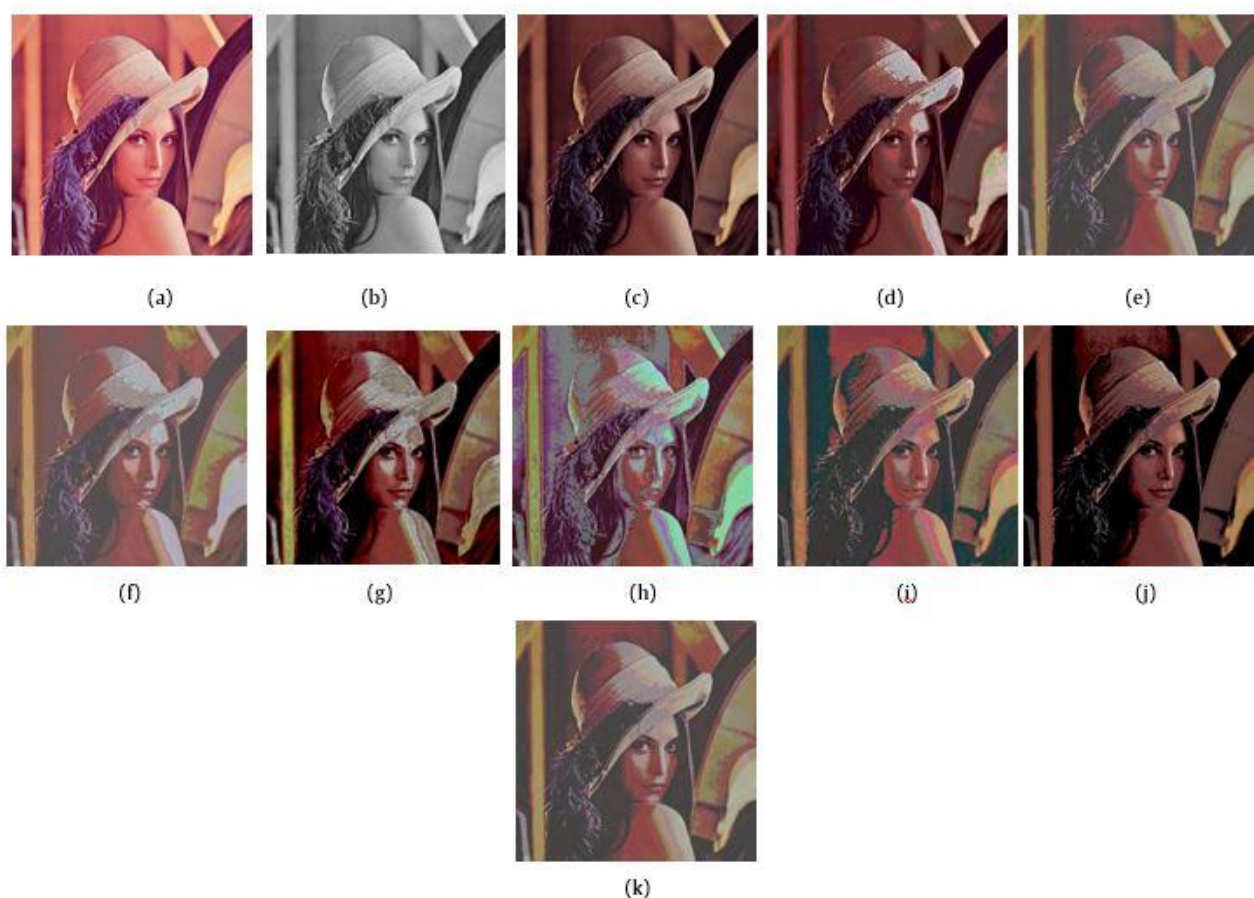
Figure 14. Image multiplication results: (a) First input, (b) Second input, (c) Exact result, (d) IFA1, (e) IFA2, (f) IFA3, (g) IFA4, (h) IFA5, (i) IFA6, (j) IFA7, (k) Minority-based IFA.
