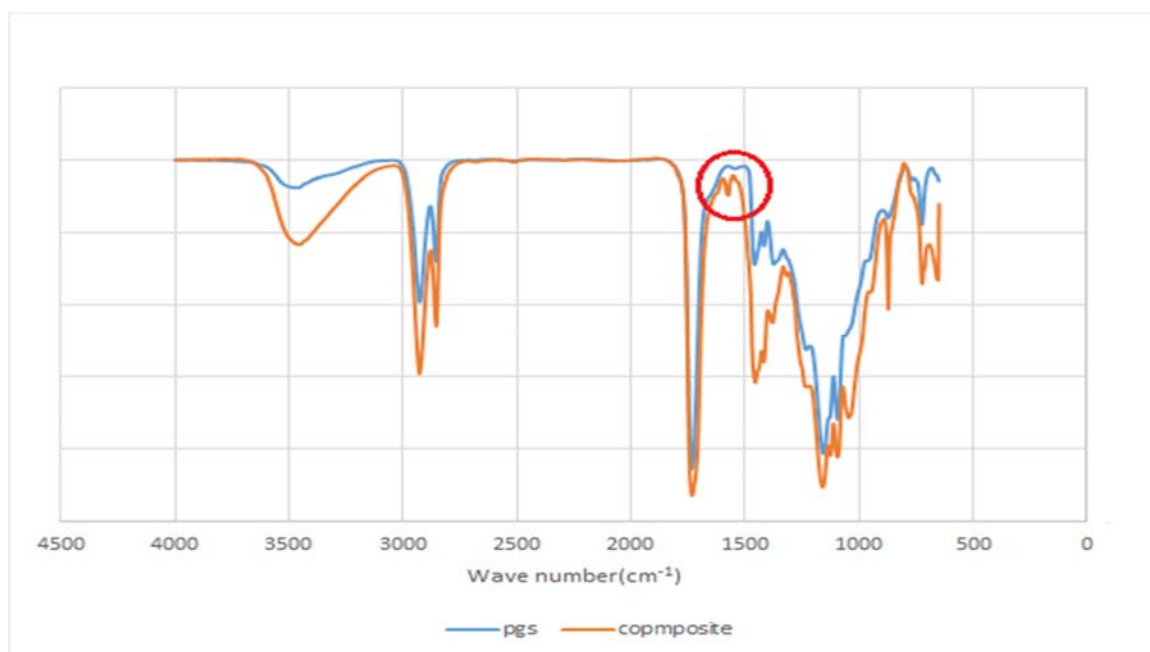
Figure 3. FTIR spectrum of PGS/CaTiO 3 in comparison to PGS. The red circle shows metallic carboxylate bond.
