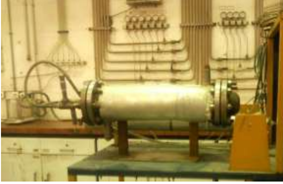
Figure 5. Experimental setup of shell & tube heat exchanger
