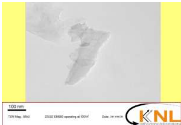
Figure 3. TEM image of graphene synthesized by CVD method
