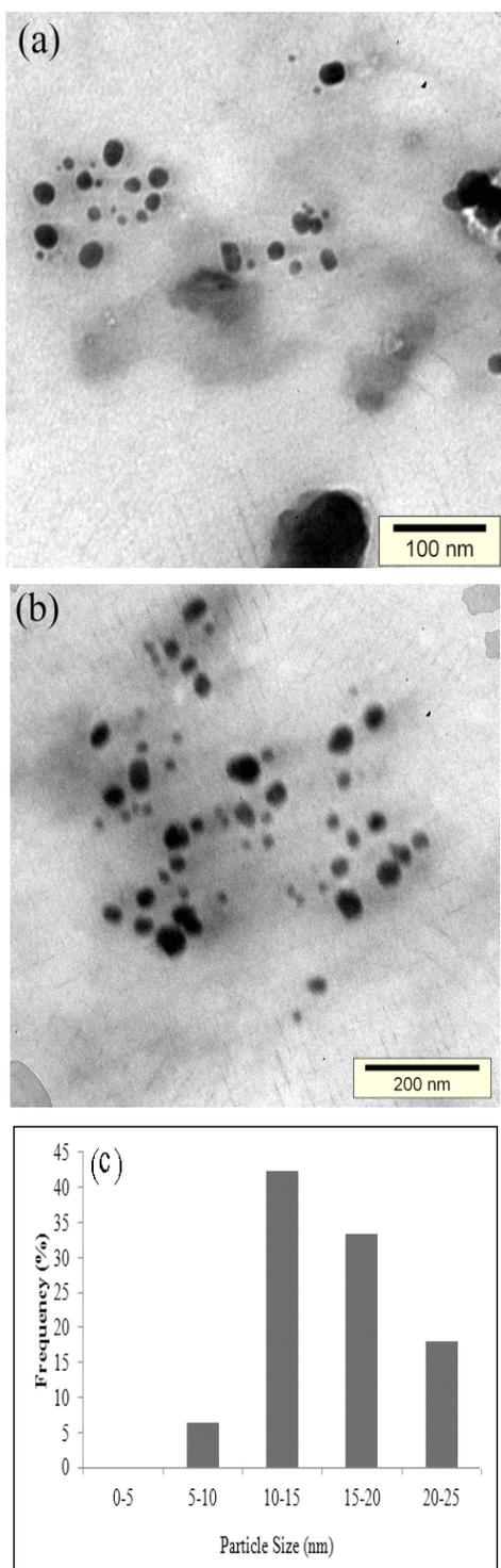
**Figure 1.** (a) TEM image of silver nanoparticles synthesized with 10% of *Lens* seed extract, 3 mM of  $AgNO_3$  incubated at 25°C for 24 h at pH 3.0; (a) magnified 40000 $\times$  (b) magnified 50000 $\times$  (c) Histogram of particle size distribution
