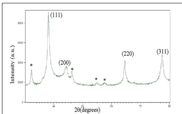
**Figure 2.** XRD pattern recorded for the nanoparticles synthesized from *Lens culinaris* seed extract (\*show unassigned peaks).
