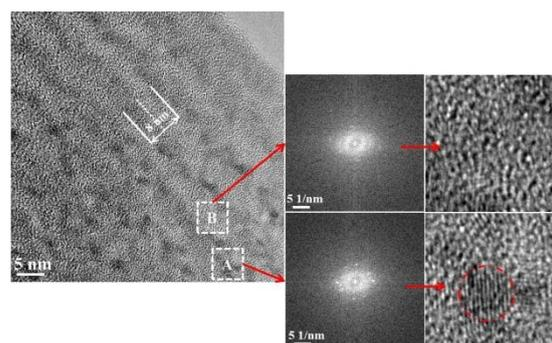
**Figure 3.** High-resolution cross-sectional TEM image of TiC/a-C:H nano-multilayer coatings deposited at 50 A arc current and the corresponding fast Fourier transformed patterns and inverse fast Fourier transform image of the selected areas A (nanocrystallite TiC layer) and B (amorphous C:H layer).
