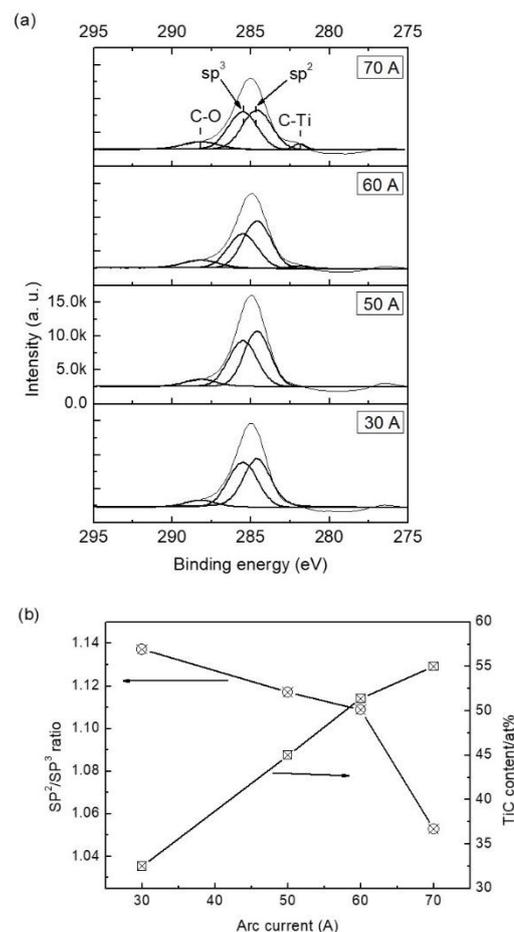
**Figure 5.** (a) XPS spectra of C1s core levels of the TiC/a-C:H nano-multilayer coatings deposited at various arc currents, (b)  $sp^2/sp^3$  ratio and contents of TiC phase at the surface of the TiC/a-C:H coatings from fitting C 1s spectra.
