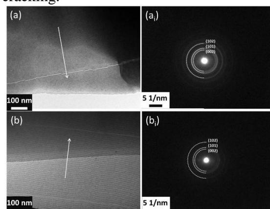
**Figure 2.** Cross-sectional TEM bright-field image of TiC/a-C:H nano-multilayer coatings deposited at arc currents of 30 A (a) and 50 A (b) and the corresponding diffraction patterns (a<sub>1</sub>) and (b<sub>1</sub>). The arrows indicate growth direction.
