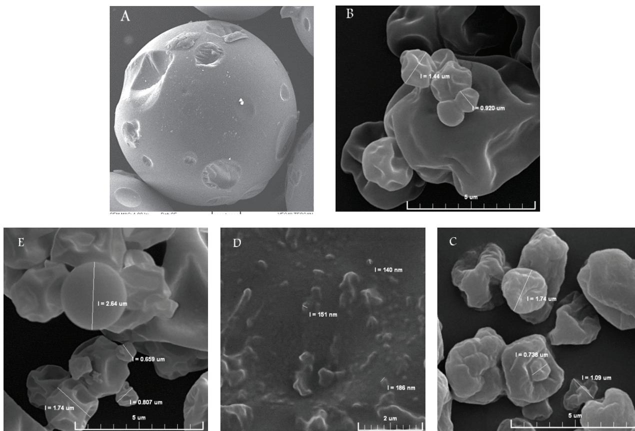
**Figure 3:** Scanning electron microscopic photographs of blueberry essential oil encapsulated powders: A:  $\beta$ -cyclodextrin(100%), B: Inulin (100%), C:  $\beta$ -cyclodextrin(50%) and Inulin (50%), D:  $\beta$ -cyclodextrin(75%) and Inulin (25%), E:  $\beta$ -cyclodextrin(25%) and Inulin (75%)
