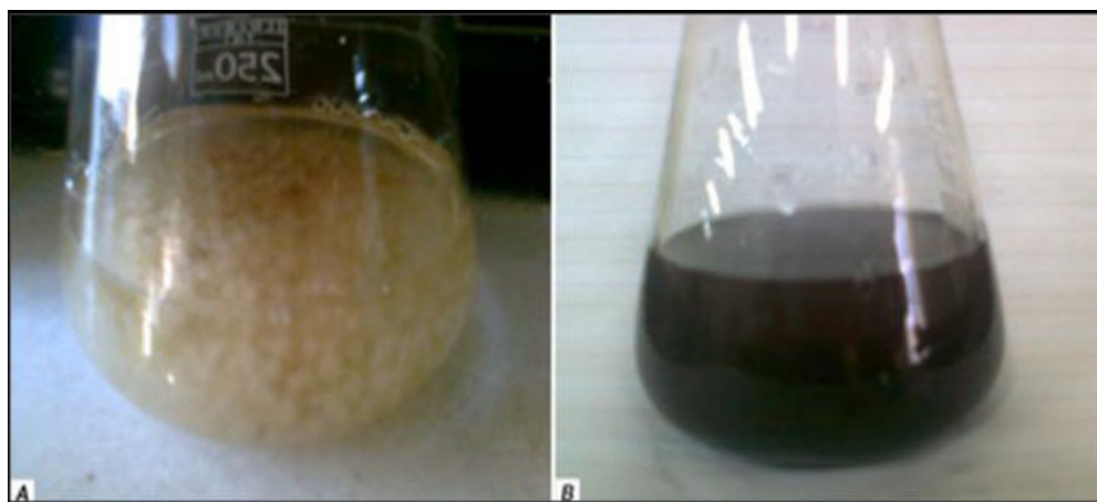
Figure 1: Penicillium chrysogenum biomass before the reaction (a) and after 12 h of the reaction (b) with the solution of 1 mM \text{HAuCl}_4 .
