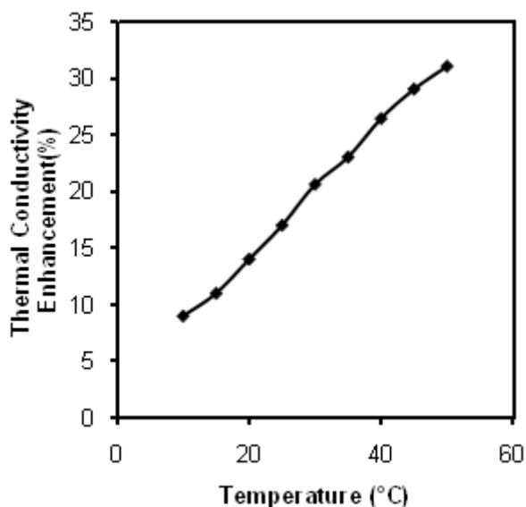
**Figure 7:** Effect of temperature on the thermal conductivity CuO-water with PVP surfactant.
