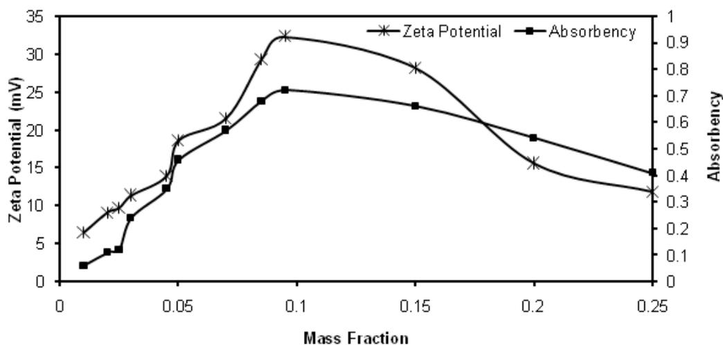
*Figure 5: Effect of PVP concentration on the zeta potential and absorbency of CuO-water.*
