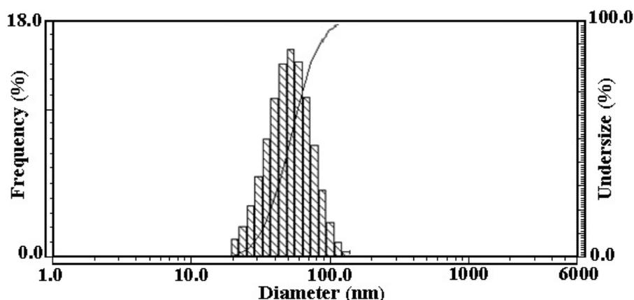
Figure 2: PSA of CuO–water nano-suspensions PVP surfactant.
