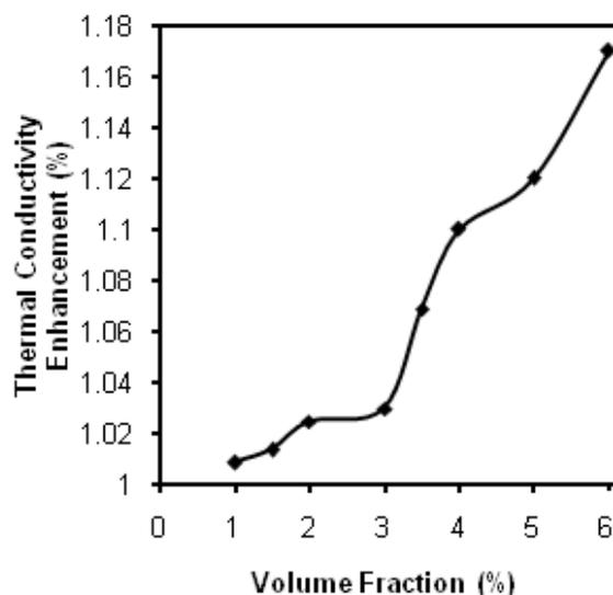
**Figure 6:** Effect of volume fraction CuO nanoparticles on the thermal conductivity of nano-suspensions with PVP surfactant.
