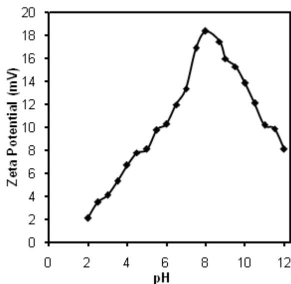
**Figure 3:** Effect of pH on the zeta potential of CuO–water nano-suspensions with PVP surfactant.
