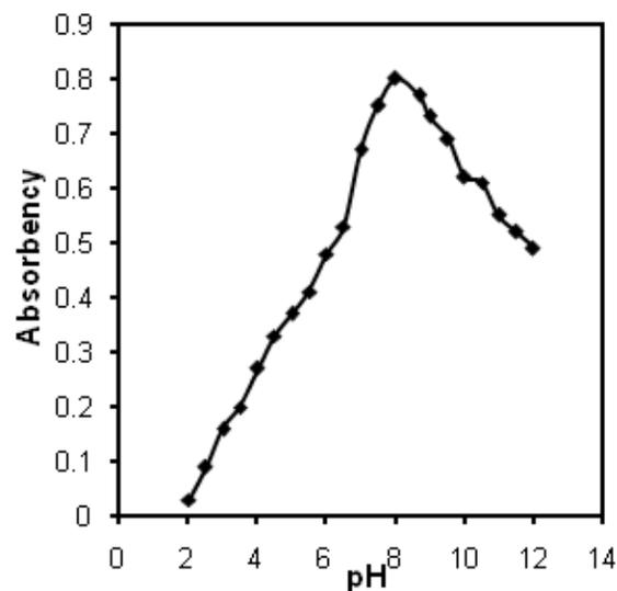
*Figure 4: Effect of pH on the absorbency of CuO–water nano-suspensions with PVP surfactant.*
