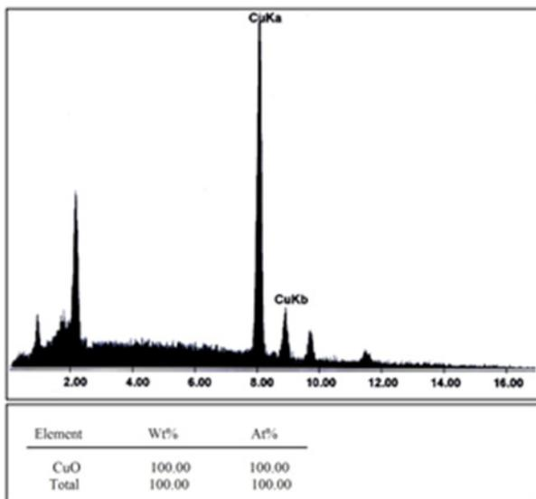
**Figure 5:** EDX analysis of as synthesized products by direct calcination of Cu(tpa)(dmf) at 400 °C.
