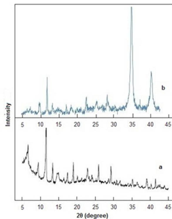
**Figure 2:** X-Ray powder diffractograms recorded for Cu-BTC; (a): reported sample; (b): as-synthesized sample.
