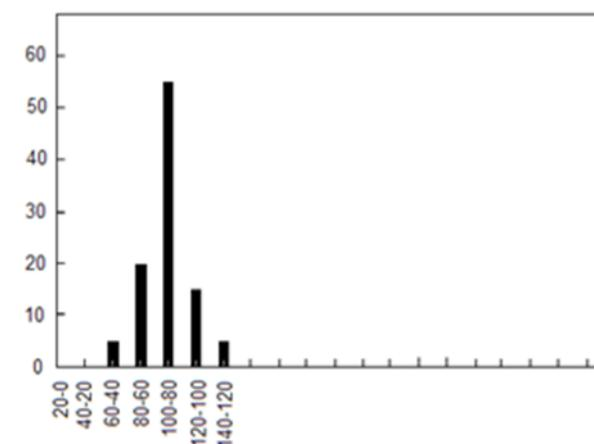
**Figure 9:** particle size histogram of  $\text{Cu}_3(\text{BTC})_2$  at 500 °C that estimated 90 nm.
