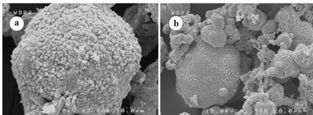
**Figure 7:** SEM photographs of copper oxide nanostructure produced by calcination of compound  $\text{Cu}_3(\text{BTC})_2$  at 500 °C.
