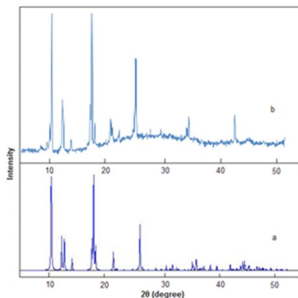
**Figure 1:** (a): XRD patterns for the simulated, and (b): as synthesized Cu(tpa).(dmf) MOF.
