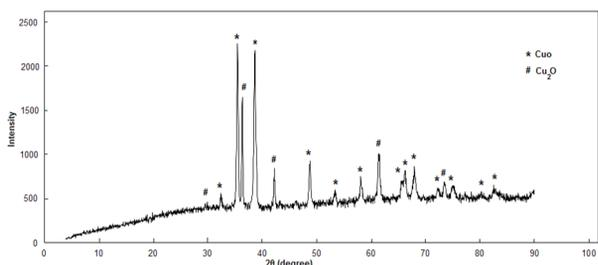
**Figure 4:** XRD pattern of as-prepared copper oxide nanoparticles after calcination of  $\text{Cu}_3(\text{BTC})_2$ .
