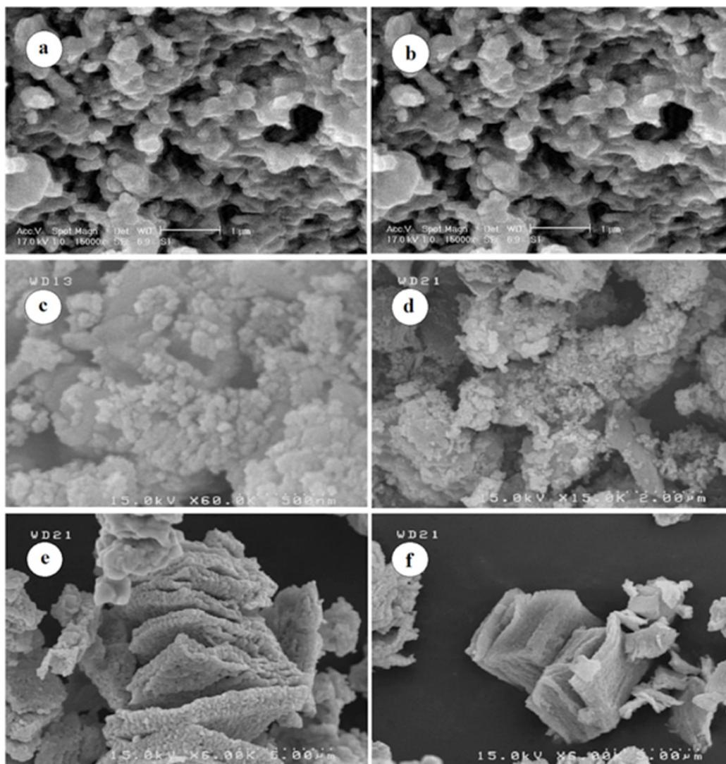
**Figure 6:** SEM photographs of CuO nanostructure produced by calcination of compound  $\text{Cu}(\text{tpa})(\text{dmf})$ ; (a-b) at 400, (c-d) 500, and (e-f) 600 °C, respectively.
