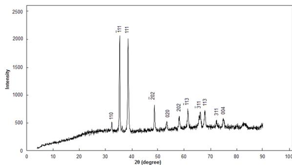
**Figure 3:** X-ray diffraction patterns of the CuO nanoparticles with tenorite structure (JCPDS no. 41-0254) by thermolysis of Cu(tpa)(dmf) MOF.
