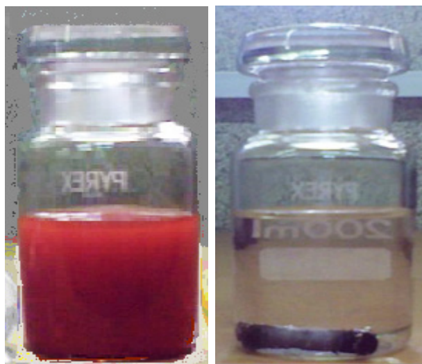
Figure 1: Solution of \text{Fe}_2\text{O}_3 (Left hand-side) and \text{Fe}_2\text{O}_3@\text{Pt} core-shell NPs (Right hand-side)
