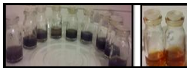
Figure 1. change in color of all samples exposed to sunlight (right); UV (left).
