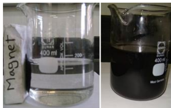
Figure 7. Separation of the Fe_3O_4@SiO_2@meso-SiO_2 particles by a magnet during 20 s.
