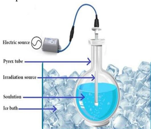
**Figure 1.** Photocell of Synthesis NiO-NPs
