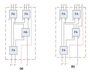
Figure 5. Implementation of (a) 6:3 Compressor, (b) 7:3 Compressor.
