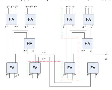
Figure 4. Cascade connection of two 6:2 Compressors.
