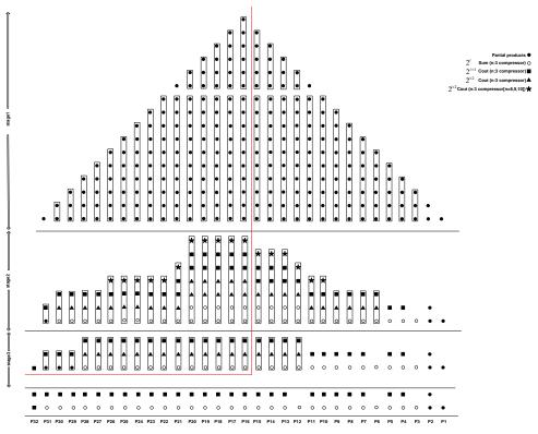
*Figure 8.* The proposed  $16 \times 16$ -bit multiplier cell using m:3 compressors.
