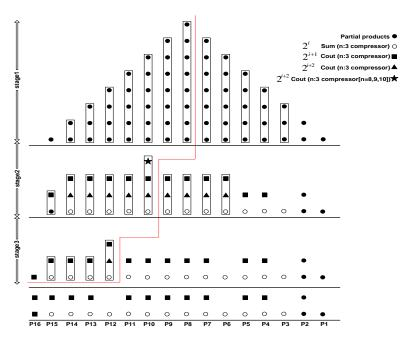
*Figure 7.* The proposed  $8 \times 8$ -bit multiplier cell using m: 3 compressors.
