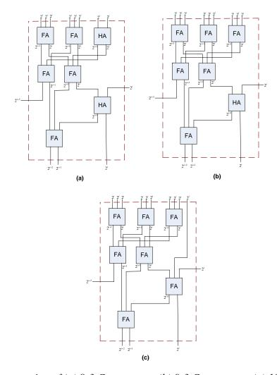
Figure 6. Implementation of (a) 8:3 Compressor, (b) 9:3 Compressor, (c) 10:3 Compressor.
