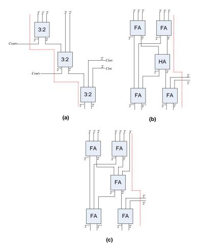
Figure 3. Implementation of (a) 5:2 Compressor, (b) 6:2 Compressor, (c) 7:2 Compressor.
