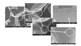
Figure3. SEM images of PUCC nanocomposite loaded with 1.0 wt% SiO<sub>2</sub> NPs at different magnification, (a) ×100, (b) × 500, (c) × 1k, (d) × 6k and (e) ×30k to show micro voids.
