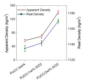
*Figure7.* Apparent and real density of blank PUCC and PUCC/SiO<sub>2</sub> NPs.
