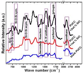
Figure 5. FTIR spectra of blank PUCC and PUCC/SiO<sub>2</sub> nanocomposites
