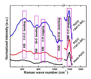
*Figure4.* Raman spectra of blank PUCC, and PUCC/SiO<sub>2</sub> nanocomposites.
