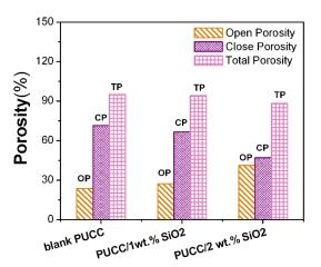
Figure8. Total porosity, open porosity and closed porosity of blank PUCC and PUCC/ SiO<sub>2</sub> NPs.
