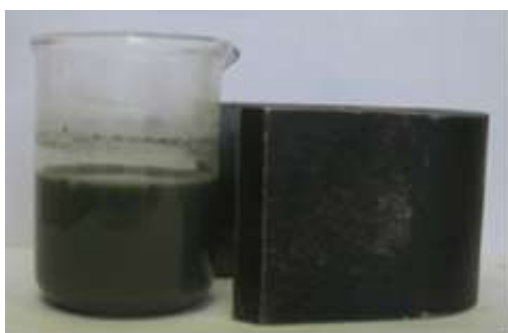
Figure 6. Coated and uncoated iron nanoparticles- the right image: uncoated iron nanoparticles are attracted to the magnet quickly; the left picture: coated iron nanoparticles show little tendency towards the magnet.
