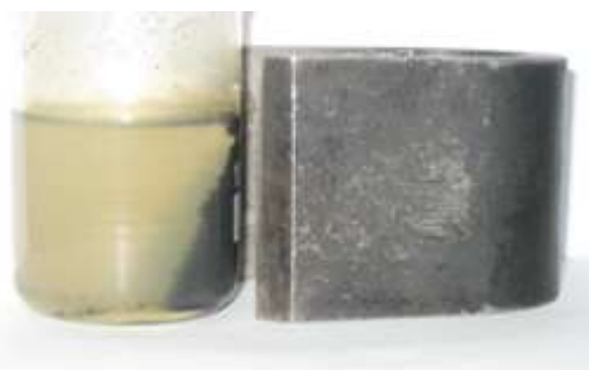
Figure 6. Coated and uncoated iron nanoparticles- the right image: uncoated iron nanoparticles are attracted to the magnet quickly; the left picture: coated iron nanoparticles show little tendency towards the magnet.
