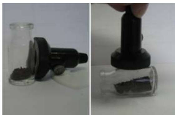
Figure 6. Coated and uncoated iron nanoparticles- the right image: uncoated iron nanoparticles are attracted to the magnet quickly; the left picture: coated iron nanoparticles show little tendency towards the magnet.
