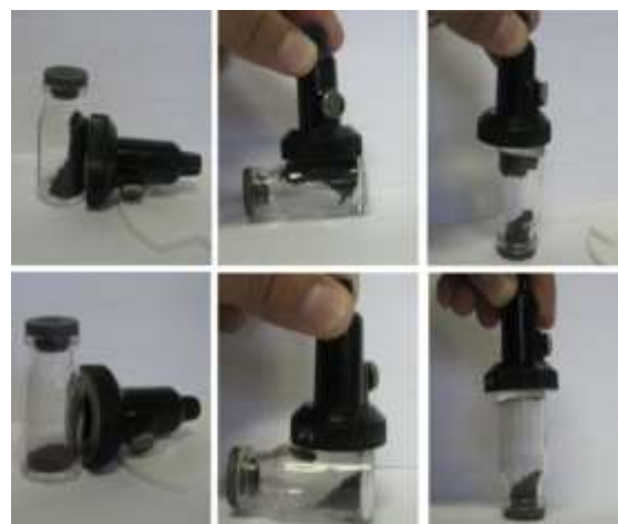
Figure 10. Visual observations of the magnetite and barium hexaferrite nanoparticle response to a magnetic field. The upper images are related to magnetite nanoparticles, and the lower pictures are related to the barium hexaferrite nanoparticles.
