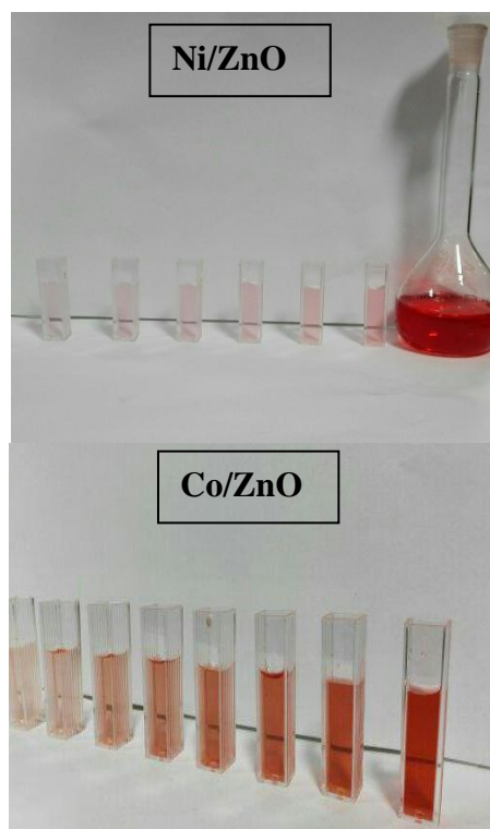
Figure 7. Congo red solutions of Co and Ni/ZnO structures after UV irradiation at different times.
