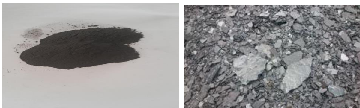
Figure 2. The oxide shell image before and after mill.
