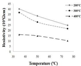
*Figure 7. Effect of both post annealing and substrate temperature on resistivity of CdS thin films.*
