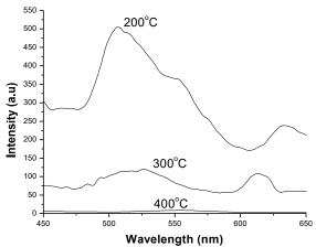
*Figure 4.PL spectra of CdS/Si thin films for different annealing temperature.*
