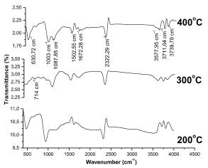
*Figure 5. FTIR* spectra of CdS/Si thin films for different annealing temperature.
