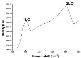
*Figure 3. Raman spectra of CdS thin films annealed at 400°C.*
