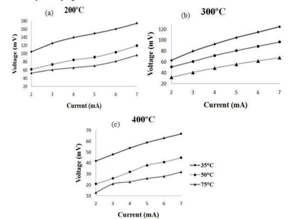
Figure 6. Voltage – Current characteristics of CdS thin films.
