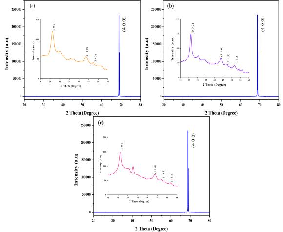
*Figure 1. XRD pattern of CdS thin films for different post annealing temperature.*
