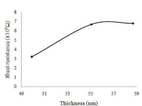
**Figure 8.** Variation of sheet resistance with thickness of CdS thin film on silicon substrates.
