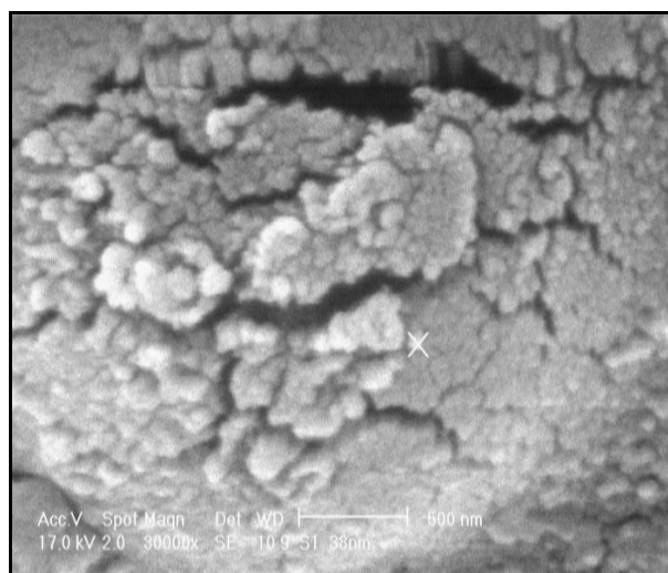
Figure 2: SEM photograph of tearing of the prepared sample in the presence of \text{CHCl}_3 as antisolvent. This tearing happens because of low thermal consistence.
